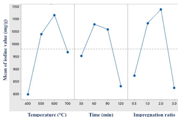
Fig. 1. Effect of temperature, time and impregnation ratio on iodine number
